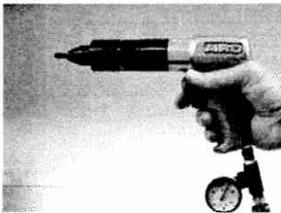
Test dynamic air pressure readings at the location where the tool is to be operated* (Instructions, Pg. 3)
